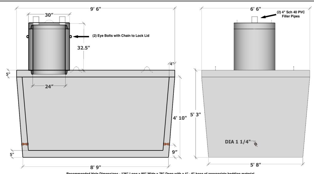
Recommended Hole Dimensions - 126" Long x 90" Wide x 78" Deep with a 4" - 6" base of appropriate bedding material When installing two or more cisterns, leave enough space between the tanks that your excavator bucket will fit for proper backfilling.
